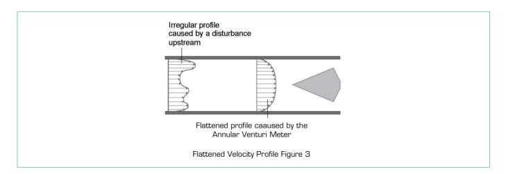
The Annular venturi meter can flatten the flow profile under even conditions, such as single elbows or double elbows out-of-plane positioned closely upstream of the meter. This means that as different flow profiles approach the cone, there will always be a predictable flow profile at the cone. This ensures accurate measurements even in non-ideal conditions.
