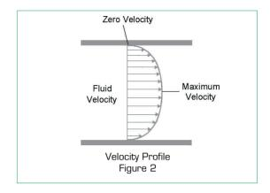
the pipe, it interacts directly with the "high velocity core" of the flow. The cone forces the high velocity core to mix with the lower velocity flows closer to the pipe walls. Other Dp meters have centrally located openings and do not interact with this high velocity core.
