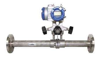
The integral orifice is a flow element capable of beingclose coupled with differential pressure transmitters tomake a complete flow meter. It provides easy-to-install, low-cost measurement of the small flows found frequentlyin plant metering operations and research projects.
